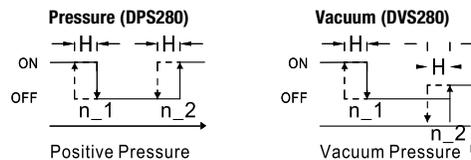
**[NOTES:]** It is recommended the Hysteresis value be set greater than the  $\pm 0.2\%$  of FS repeatability. If set lower and the applied pressure fluctuates too near the set point, it can cause the digital output to chatter.
