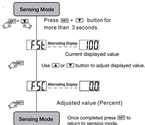
To enter fine adjustment mode simultaneously press and hold **SET** +  $\blacktriangledown$  for 3 seconds.
