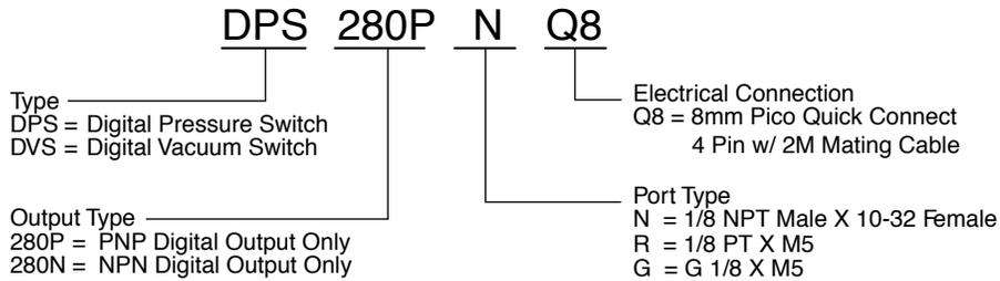
Example: DPS280PNQ8 = Digital Pressure Switch - PNP - 1/8 NPT - 8mm Pico 4 Pin w/ 2M Mating Cable
