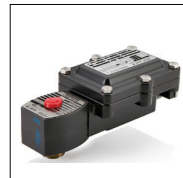
TYPE 08: Epoxy moulded, aluminum junction box, Type 7/9 JBEF : Class I, Division 1, Groups B, C, D, Class II, Division 1, Groups E, F, G
